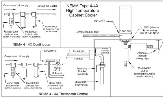
High Temperature Cabinet Coolers are rated for a maximum temperature of 200°F (94°C)
