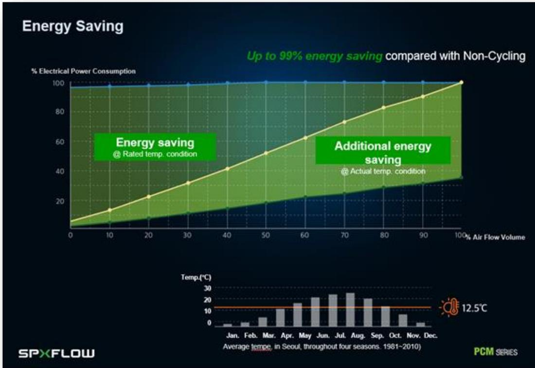
There is extra advantage with the **SPX PCM** dryer when it is operating under low ambient condition. We have tested the dryer at 15 °C ambient temperature, it draws less power compared to operating under 38 °C at the same inlet flow.
