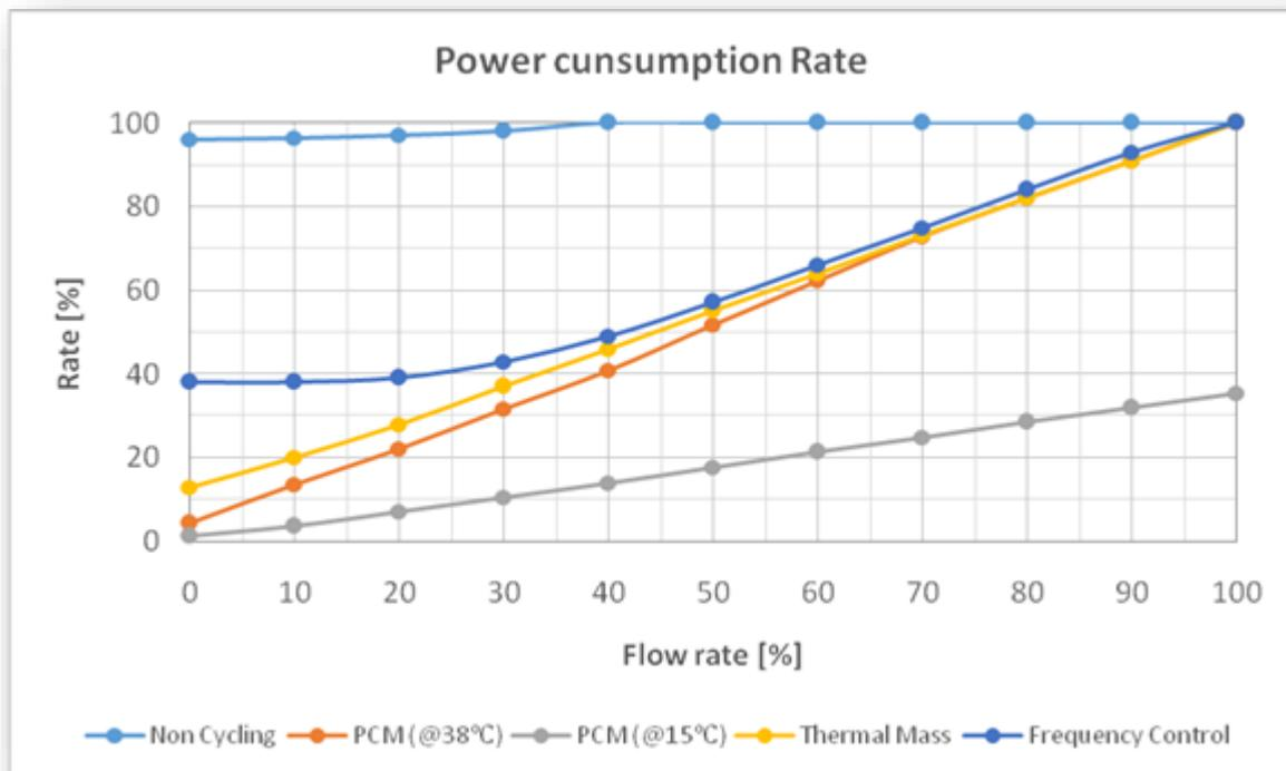
The above chart shows energy consumption of different types of refrigerated dryer.
