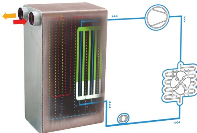
**SPX PCM** dryer's stainless steel brazed plate heat exchanger is manufactured at its own Stainless Steel BPHE manufacturing facilities in Busan, enabling full quality control internally.
