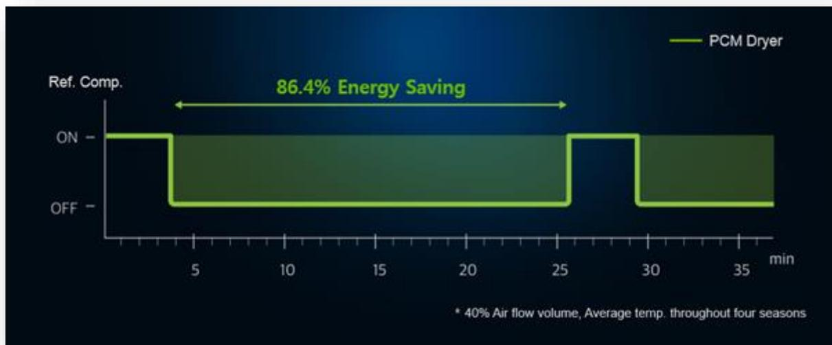
When the phase change material (**PCM**) solidifies, the refrigerant compressor stops.
