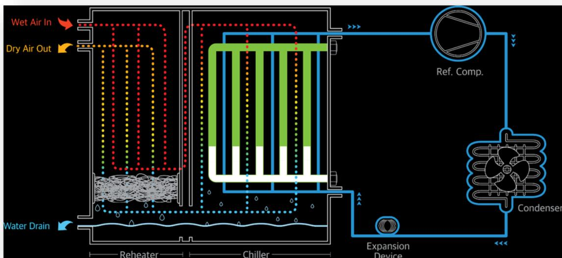
1. Compressed air saturated with water vapour enters the stainless steel brazed plate air-to-air heat exchanger. It is pre-cooled by the outgoing chilled air, and then directed to the stainless steel brazed plate **PCM-to-Air** heat exchanger (evaporator) where it is further cooled by the innovative Phase Change Material ( **PCM** ).
